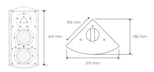
Power handling, IEC268: Power handling, peak: Sensitivity, 2,83V/1m: Maximum SPL, long term: Maximum SPL, peak: Frequency response: Nominal impedance: Dispersion: Weight: Measurements: 100 watt 400 watt 88 dB 108 dB 114 dB 59-25.000 Hz 8 ohm 120x120 degree 4,1 kg 441x213x154mm
