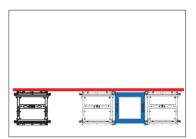
4.3 Using the small spacer, place the first wall mount of the next row.
