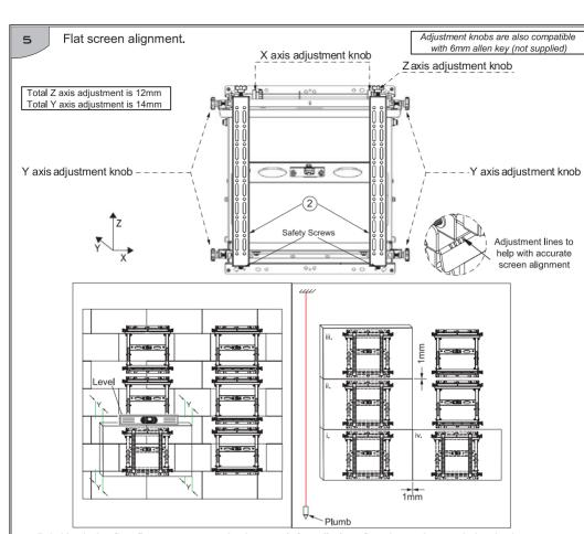
5.1 Hook the first flat screen onto the bottom left wall plate first. keep the x axis knobs between the middle of the two interface arms (part 2).
