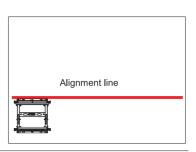
4.2 Using the large spacer, place the second wall mount as shown whilst being careful to keep on the alignment line.
