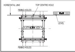
2.3 Fix the wall mount to the wall (use the horizontal line as a guide), using the fixing holes with suitable wall fixings (not supplied).
