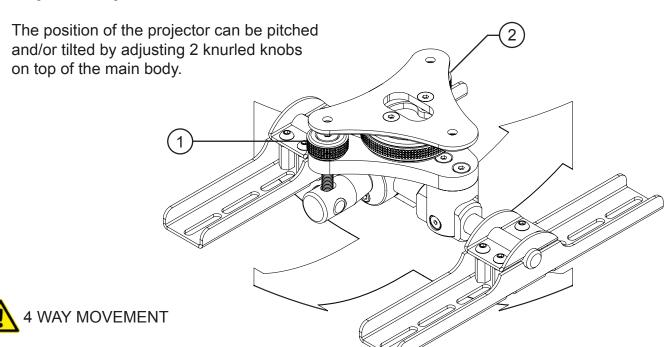
Rotate both knobs in SAME DIRECTION to adjust TILT Rotate both knobs in OPPOSITE DIRECTION to adjust PITCH
