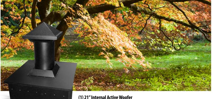
The 211ST 21" subterranean subwoofer was developed for high SPL bass output outdoor applications. In features a powerful 21" transducer for maximum excursion and SPL. There is no 70V version though it can be used as a 70V sub by being driven by an M1000 subwoofer amp which produces 70V output. No 70V transformers are used in the 211ST even for 70V application. All applications should be bi-amped.
